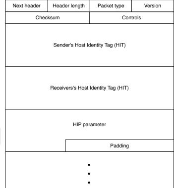
Fig. 3. HIP control packet format.
